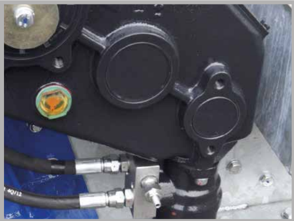
Blow off valve
