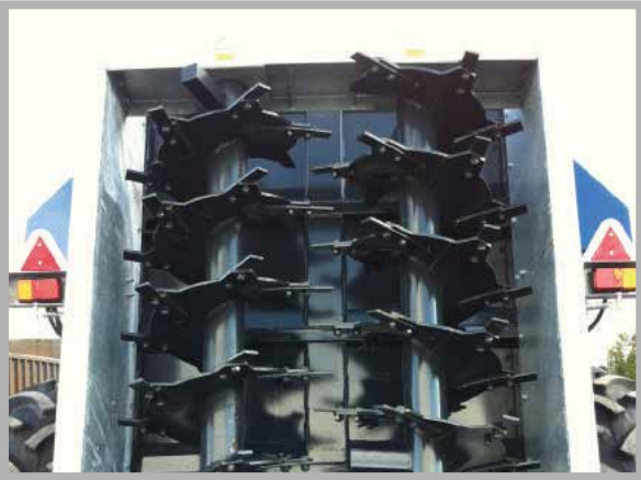
Dynamically balanced twin vertical beaters
