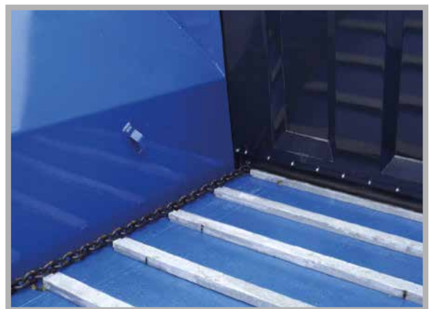
Galvanised floor lats
